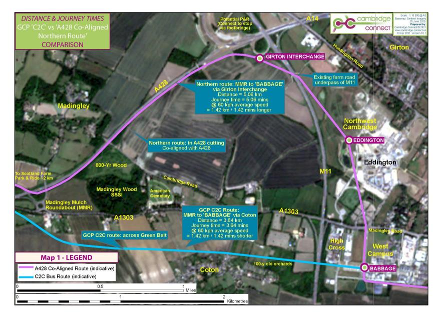
Figure 1. A428 alternative C2C alignment – co-aligned with the A428 in section from Madingley Mulch to West Campus overview.
