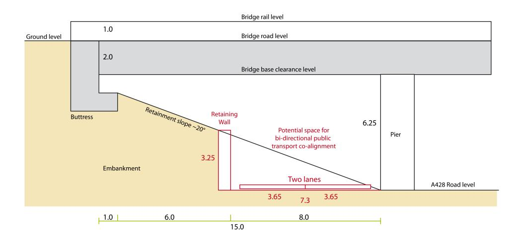
Madingley dimensions - 15.0 m from pier to buttress edge, 6.25 m height from A428 road level to clearance under bridge. Church Road dimensions - 16.0 m from pier to buttress edge, 8.0 m height from A428 road level to clearance under bridge. A428 MMR Offramp dimensions - 15.0 m from pier to buttress edge, 5.0 m height from A428 road level to clearance under bridge.
